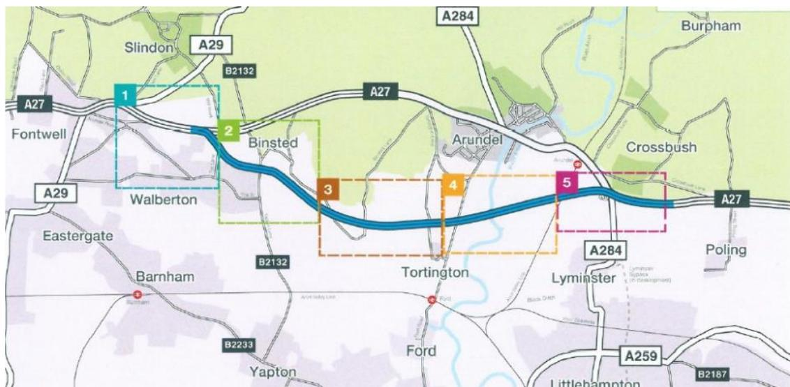
The Grey route is shown above and is an 'off-line' solution. It runs from the existing Crossbush Junction, in the east (although the junction will be remodelled), over the railway line, crossing the River Arun and its flood plain on a viaduct. It then passes to the south of Binsted Wood, through part of the Avisford Golf Course, crossing Tye Lane, to reconnect with the existing A27 around Copse Lane, Walberton.
